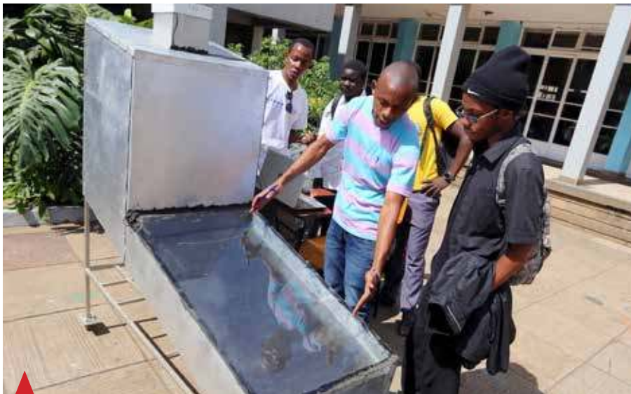
Mr. Bernard Mwashighadi and Mr. Lawrence Githinji both 5 th year Mechanical Engineering students showcase a mango solar drier which they made. The innovation is a milestone for increasing the shelf life of mangoes.
